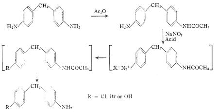
The first step in the synthesis involves the monoacetylation of 4,4'-diaminodiphenylmethane with acetic anhydride in dilute alcoholic hydrochloric acid solution in 35-43% yields. Considerable unchanged 4,4'-diaminodiphenylmethane
